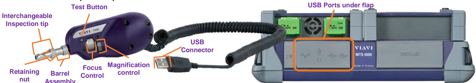
Figure 3: P5000i and T-BERD/MTS 4000 V2
